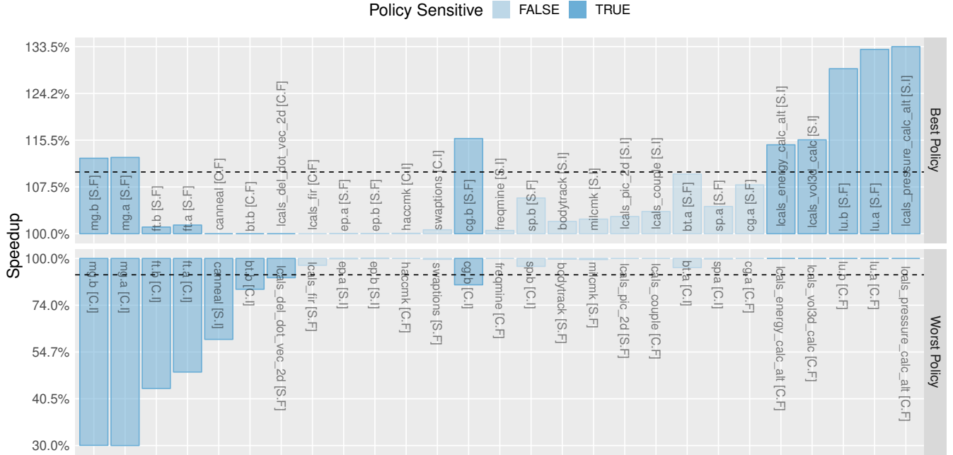
Figure 2: Application speedups with best- and worst-placement policies and placement sensitivity on the Skylake platform. Policies are noted [thread policy, data policy], with C for Compact, S for Scatter, F for Firsttouch, and I for Interleave.
