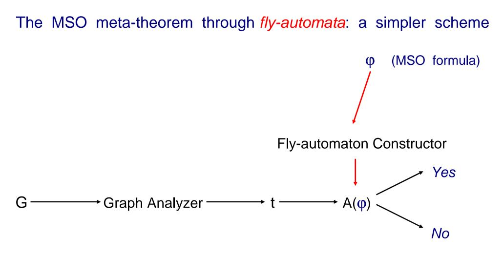
A( $\phi$ ): *infinite fly-automaton* over the countable set of all graph operations that define clique-width. The time taken by A( $\phi$ ) depends on the labels that occur in t, not only on the size of G or of t.
