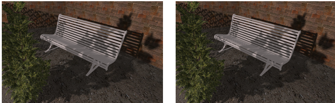
Figure 1: A scene including alpha-textured meshes (foliage and wire netting). Left: illustration of realistic soft shadows produced by the average of 1024 hard shadows (2.5s per frame). Right: our new soft shadow algorithm rendering the same scene at 25 fps without any precomputation.
