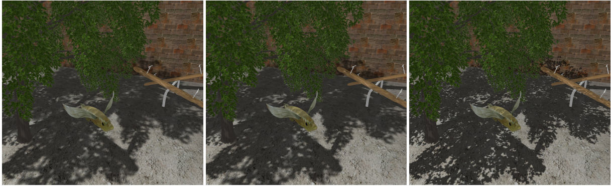
Figure 8: A scene composed of 800k polygons (screen resolution: 768 \times 768 pixels). From left to right: reference image obtained from the average of 1024 light samples (17s per frame), our algorithm without adaptive resolution (23 fps) and standard shadow mapping with hardware 2 \times 2 percentage closer filtering showing the pixels of the shadow map (40 fps).
