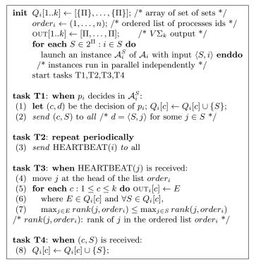
Figure 1: Emulation of  $V\Sigma_k$  from an algorithm  $\mathcal{A}$  that uses a failure detector  $\mathcal{D}$  to solve k-parallel consensus (code for  $p_i$ )
