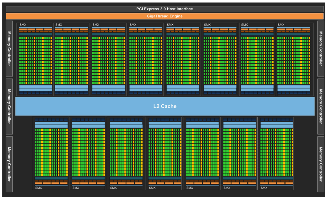
Figure 1.3 – Architecture of the NVIDIA Kepler GK110.
