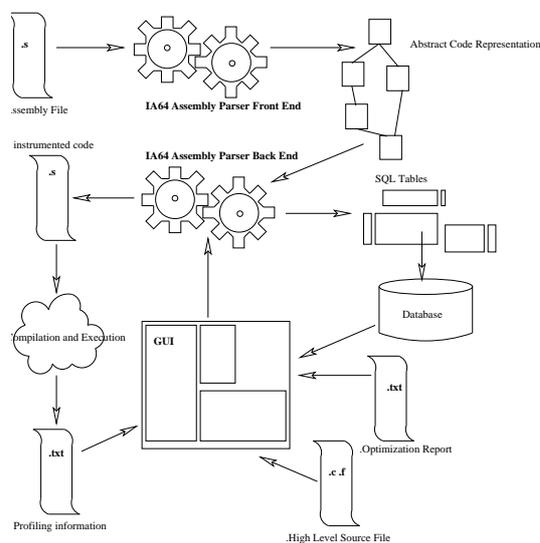
Figure 1: Overview of the assembly tool MAQAO.
