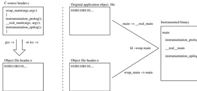
Figure 4: Overview of the wrapper: `main` from the original code is substituted with header `main` which performs memory allocation for statistics gathering and call a function to build the summary of these collected data.
