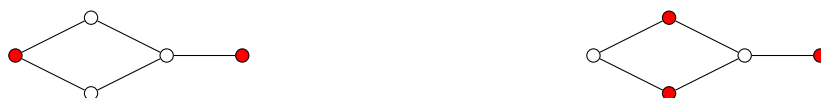
Figure 2.1: Example of a maximal (left) and a maximum (right) independent set on the same graph.
