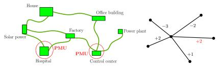
Placing a minimal number of measurement units (PMUs) to monitor an electrical system (devices and cables):
