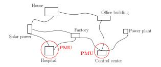
Placing a minimal number of measurement units (PMUs) to monitor an electrical system (devices and cables):
