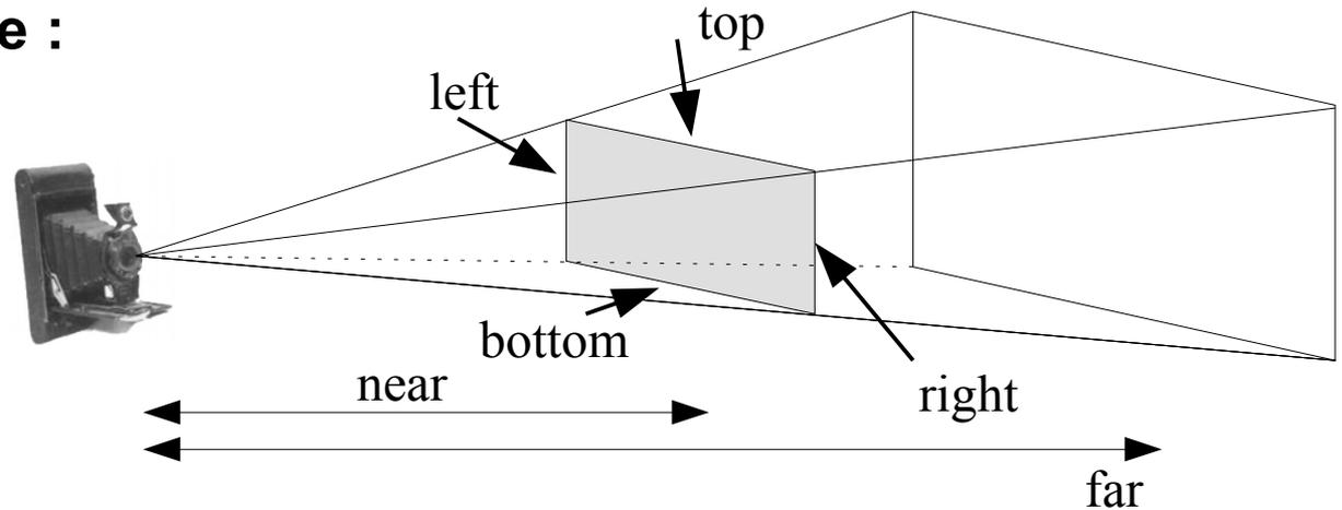
$$\begin{pmatrix} \frac{2n}{r-l} & 0 & \frac{r+l}{r-l} & 0 \\ 0 & \frac{2n}{t-b} & \frac{t+b}{t-b} & 0 \\ 0 & 0 & -\frac{f+n}{f-n} & -\frac{2fn}{f-n} \\ 0 & 0 & -1 & 0 \end{pmatrix}$$
