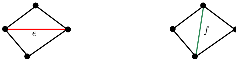
Figure 1.29 – Example of flip: the diagonal e is replaced by the other diagonal f .
