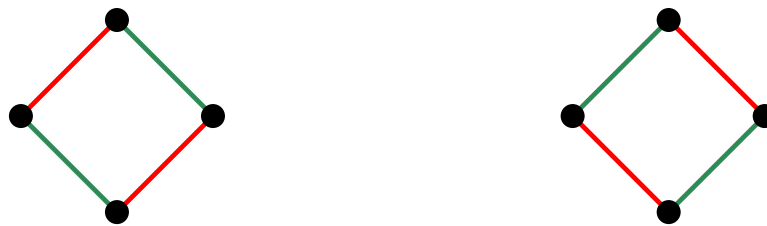
Figure 1.32 – Example of flip: the green edges are edges of a perfect matching M and the red ones are edges of another perfect matching M' .
