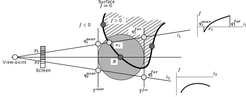
Figure 2: The projection of a sphere to the screen in 2D.
