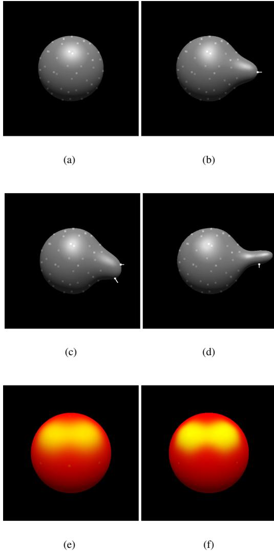
Figure 3: Modelling on a sphere. (a) Starting points, (b) moving a point, (c) adding a point, (d) changing a normal, (e)-(f) changing point materials.
