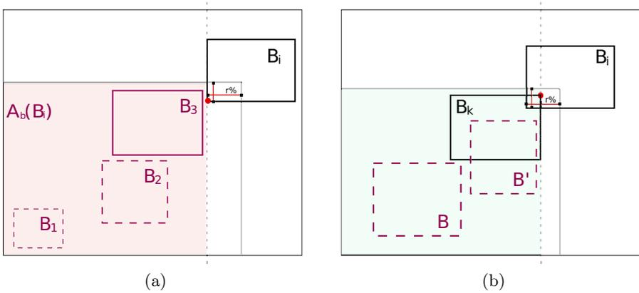
**Fig. 2.** (a) When the sweep line passes  $l(B_i)$ ,  $\text{Pred}[B_i]$  is a partial optimum on the set of possible predecessors of  $B_i$  lying in  $A_b(B_i)$ . In the example,  $B_3$  is the best current predecessor of  $B_i$ . (b) When the sweep line passes  $u(B_k)$ ,  $\text{Pred}[B_i]$  is a partial optimum on the set of possible predecessors of  $B_i$  from  $A_b(B_i) \cup \{B \in A_o(B_i) / P_1(u(B)) < P_1(u(B_k))\}$ .
