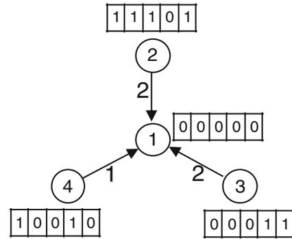
Fig. 4 Example of the optimal chunk scheduling problem
