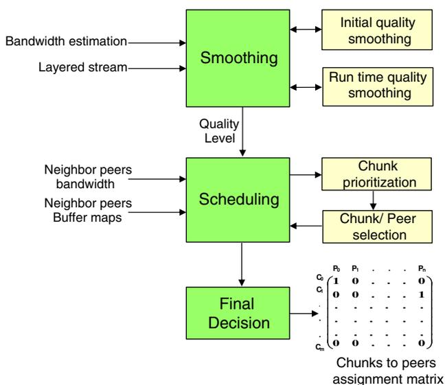
Fig. 7 Workflow of proposed playout smoothing mechanism
