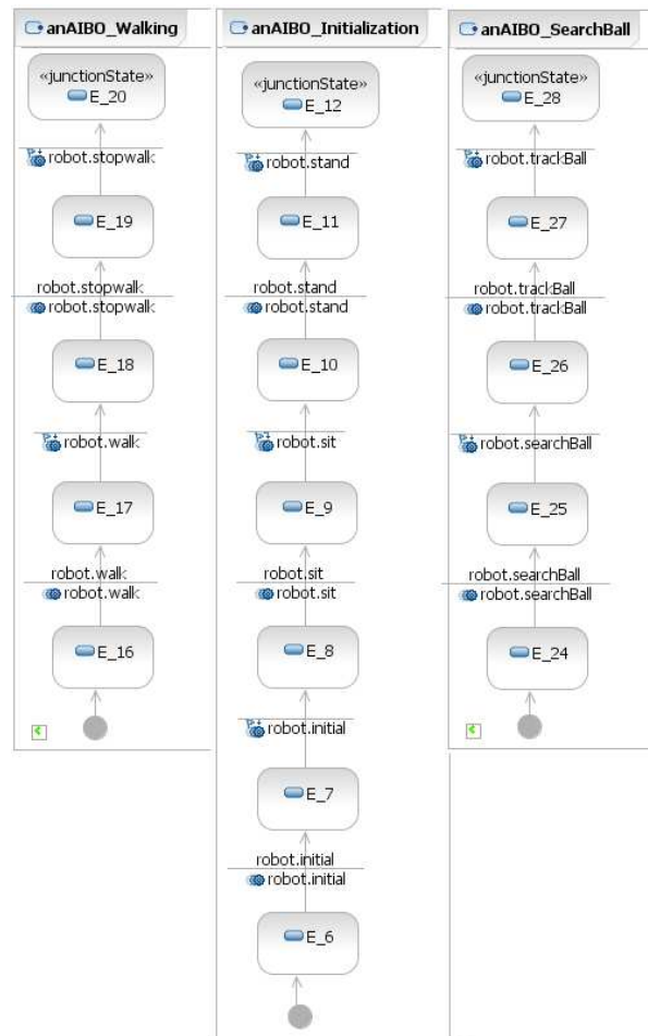
Figure 6. State machines for the AIBO object
