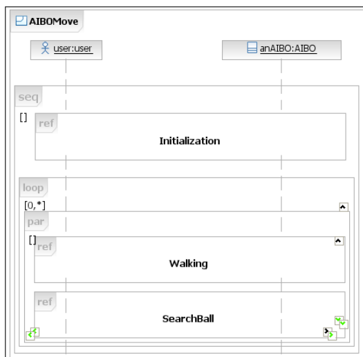
Figure 3. A Combined Sequence Diagram
